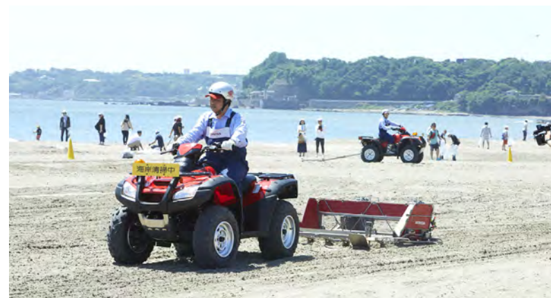
Honda Beach Cleaner that can dig up and collect trash in the sand.
