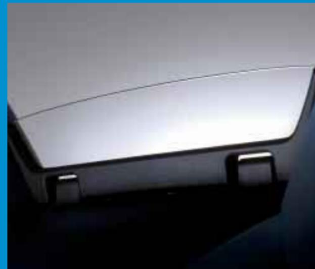
*Turbulence in the cabin is reduced, due to the folding wind deflector, located between the headrests.*
