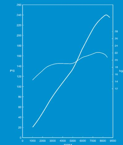
*The Honda DOHC VTEC engine combines low rev torque with high end power*
